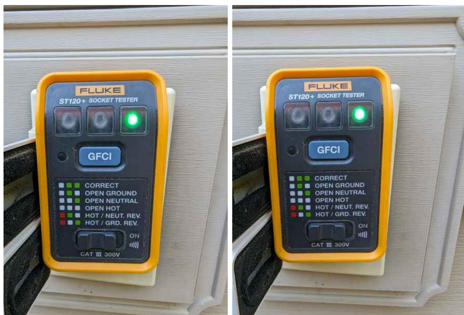
Photo error causes lights to not show up on film on occasion Outlets are wired correctly
